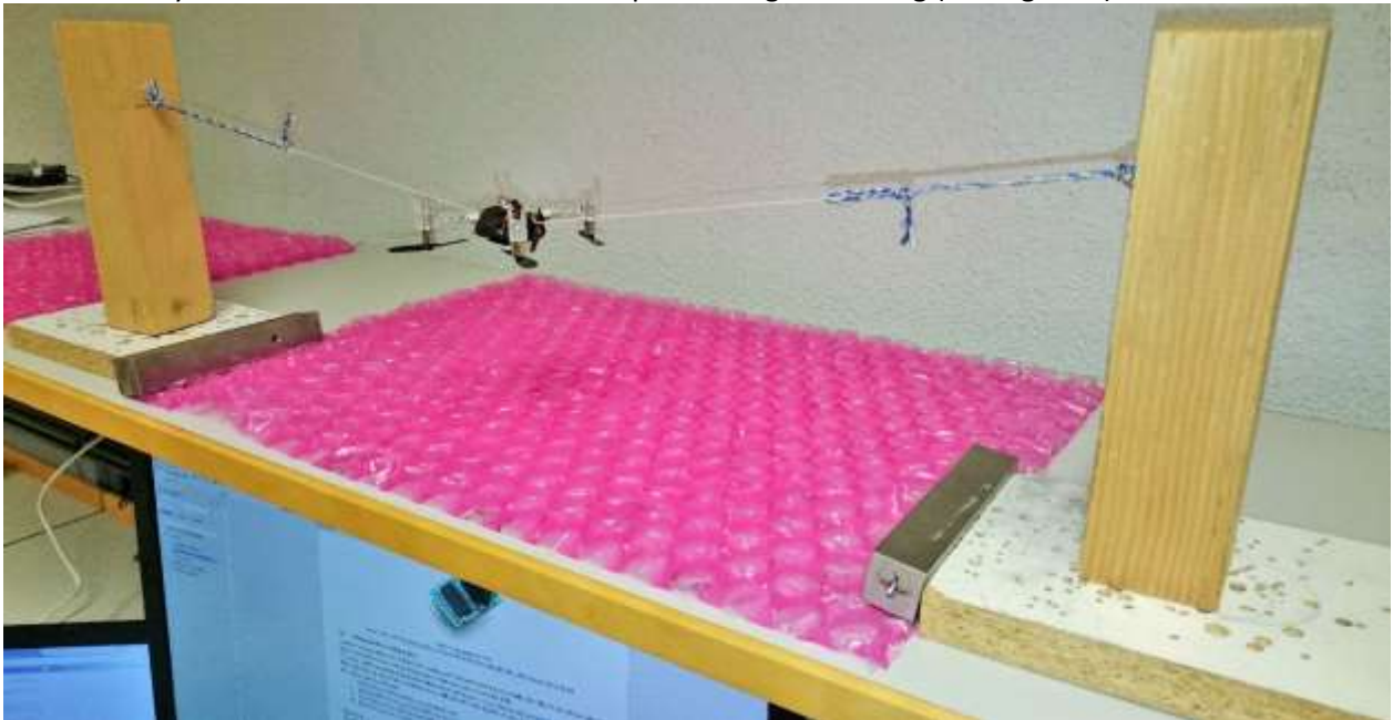
Figure 1: Support to hold still the drone when performing PID tuning.
